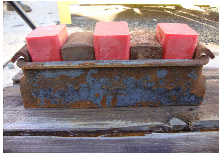
FIG. 2.3 COMPACT COLUMN SIDE BEARING Replacement cages are ordered by specifying preload, i.e. CCB6000XT Cage, where 6000 = preload, XT for extended travel. Also available in 2200lb & 3000lb preload. The 2200lb & 3000lb models are not for interchange service.
